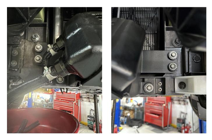
16. Once the cooler is mounted in place, we can go ahead and connect the two oil lines, the longer line goes to the connection closer to the wheel. Secure both lines with the OEM clamps.
