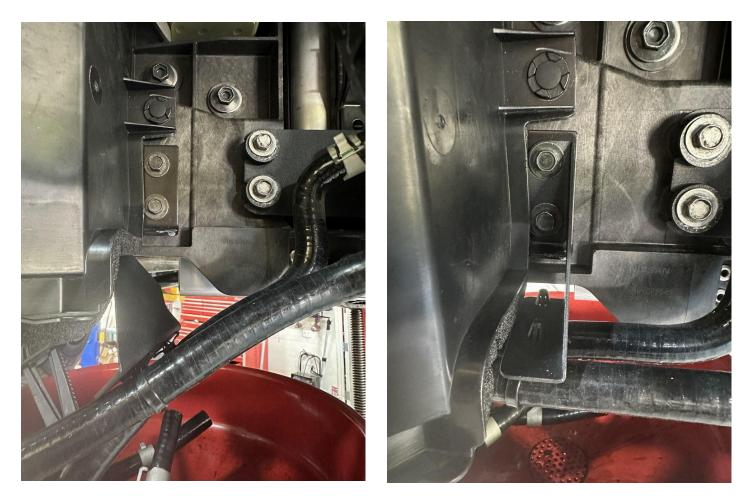
18. The upgraded oil cooler should now be fully mounted, with the lines connected and secured. We can now remove our two hose pinchers or begin refilling the car with oil, depending on which route you took.
