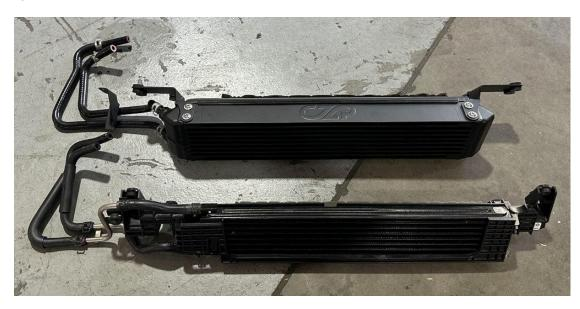
15. Now that the cooler is fully assembled and resembles the stock cooler with duct, lines, and brackets, we can go ahead and install it using the original six 10mm hex head bolts. (Torque spec is 49 in-lb or 5.5 N-m)
