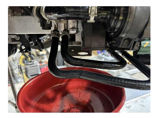
17. With the lines connected and the cooler mounted, our final piece to mount is the line support bracket which piggybacks off of the two auxiliary coolant pump mounting bolts. (Torque spec is 49 in-lb or 5.5 N-m) If you haven't done so yet, clip the lines to the bracket using the supplied ziptie style mounting clips.
